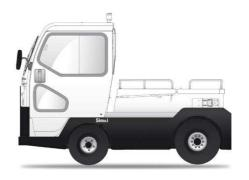
4-wheel tow tractor, man on board, with rear-wheel drive. Ideal for all intense duties - both indoors and outdoors. Loading capacity of wide rear platform 200 kg.
